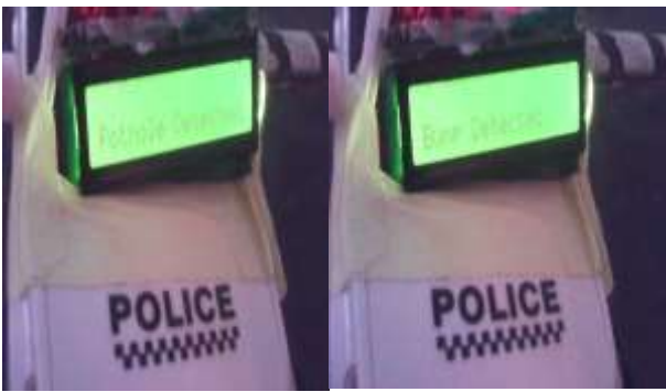
(a) Received Pothole (b) Received Bump
