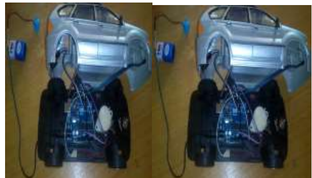
(a) Transmitter Model (b) Receiver Model Plate 2: The Development Process of both the Transmitter and Receiver Model Vehicle
