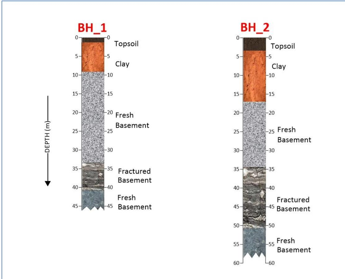
**Figure 12:** Lithological Log for borehole BH\_1 and borehole BH\_2.
