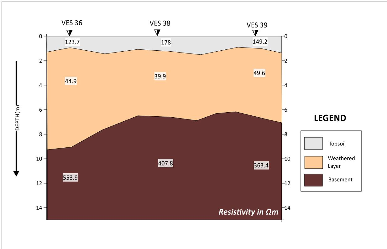
Figure 5: Geo-electric Section of Traverse 1.
