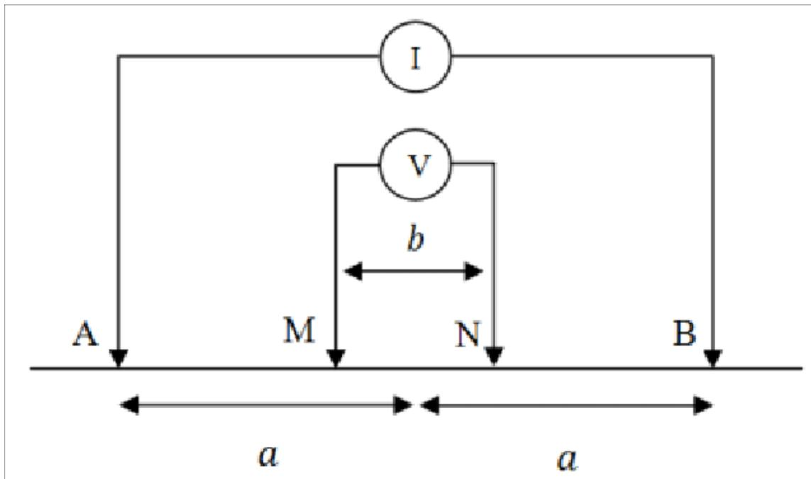
**Figure 3:** Field diagrammatic illustration of Schlumberger array configuration.
