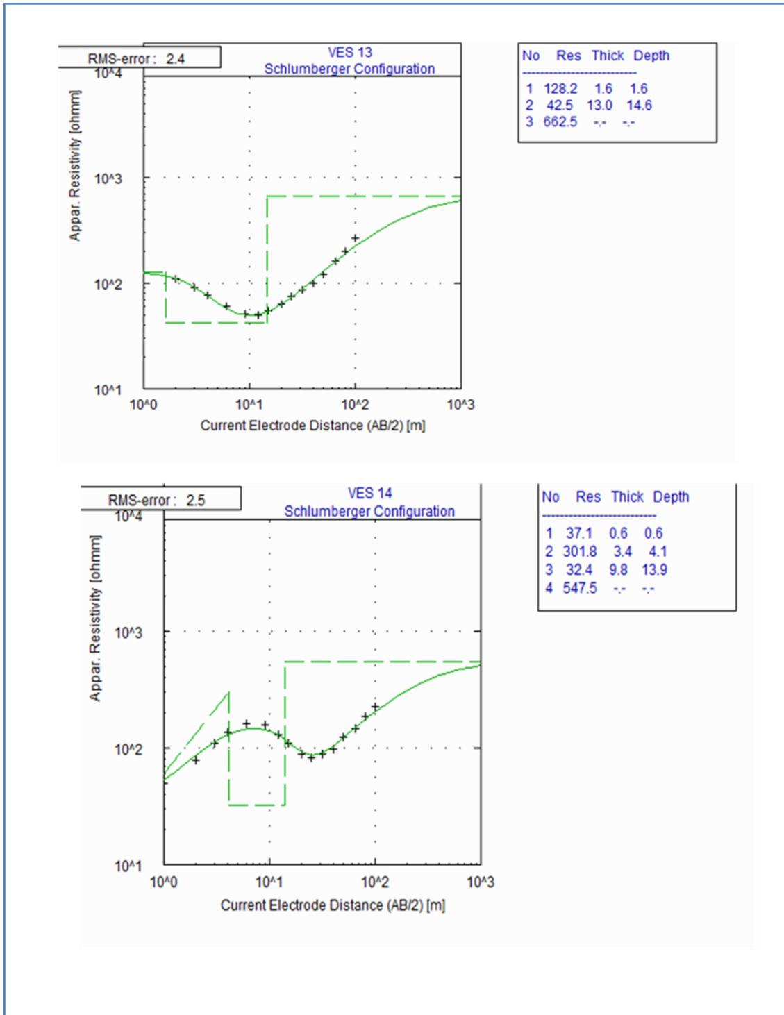
Figure 4: Iterated geophysical curve of VES 13 and VES 14 which are typical H and HK curve respectively.
