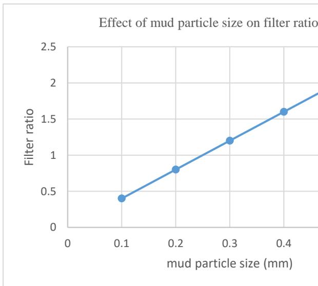
**Figure 2:** Graph of mud size particle against filter ratio.
