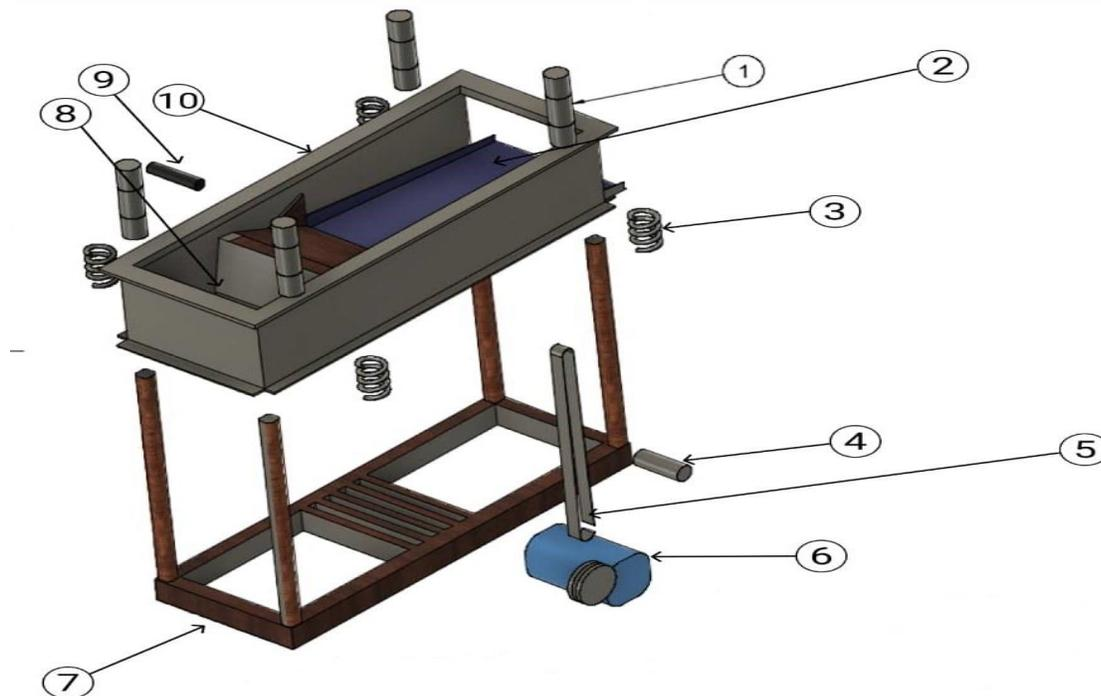
**Figure 1.** The shale shaker schematic design
