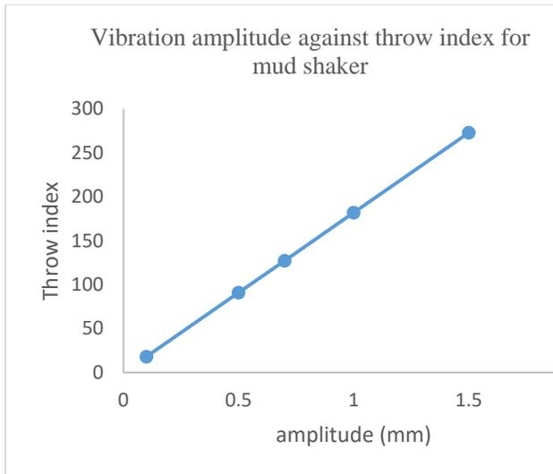
**Figure 4:** Graph of amplitude against mud particle throw index
