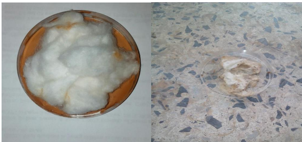
Plate I (a & b): Cotton wool wastes before and after degradation by Aspergillus niger .
