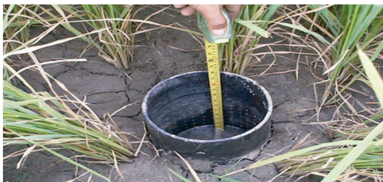
Figure 5: Safe Alternate Wetting and Drying (SAWD) Method of Irrigation
