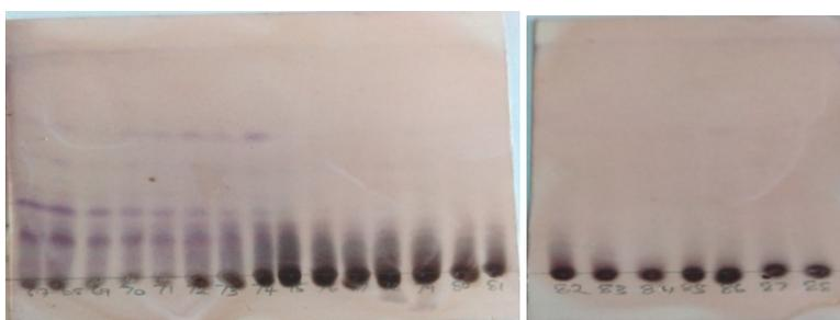
**Plate III: Column Fractions 67 to 88 of n-Hexane Fraction from Methanol Extract of *Vernonia cinerea* Developed in Hexane: Ethyl acetate (8:2) and sprayed with *p*-anisaldehyde**
