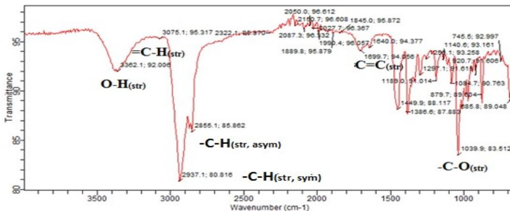
**Figure 3.1: FTIR Spectrum of VC3 with Absorption Peaks at Various Regions**
