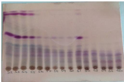
**Plate II: Column Fractions 52 to 66 of n-Hexane Fraction from Methanol Extract of *Vernonia cinerea* Developed in Hexane: Ethyl acetate (8:2) and sprayed with *p*-anisaldehyde**
