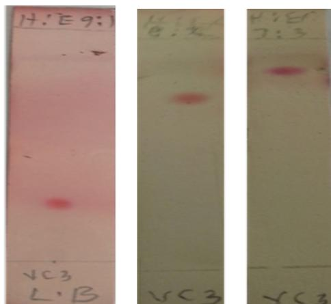
**Plate VI: TLC of VC3 from n-Hexane Fraction developed in Hexane: Ethyl acetate (9:1, 8:2 and 7:3) and sprayed with Leibermann Burchard**
