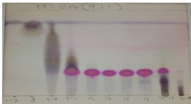
**Plate V: TLC plate for Purification of HF developed in Hexane: Ethyl acetate (9:1) and sprayed with Liebermann Burchard**
