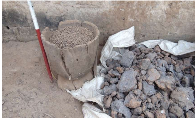
Plate III: Lumps of fired clay with the pounded grog in a mortar
