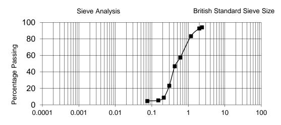
Figure 1: Sieve analysis for the fine aggregate
